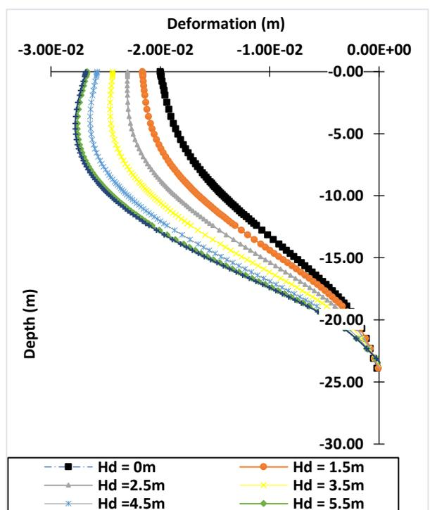
Figure 16: Deformation vs Depth of DW at ( $H_e=5m$ )
