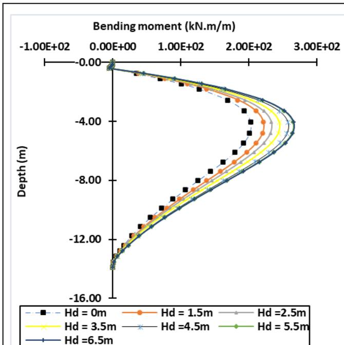
Figure 17: B.M vs Depth of barrette at ( $H_c=5m$ )
