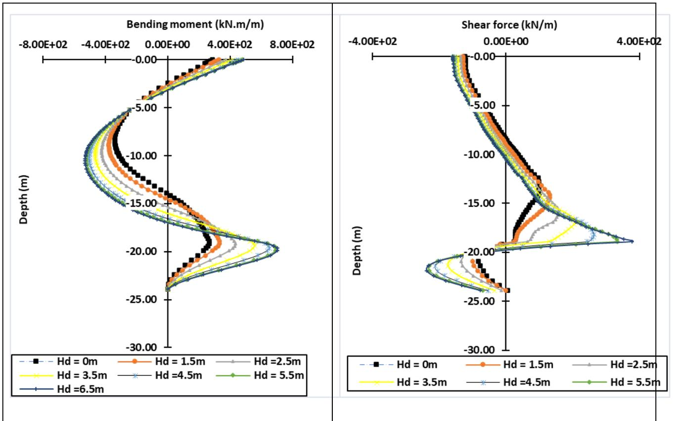
Figure 23: B.M vs Depth of DW at ( $H_e=5m$ )
