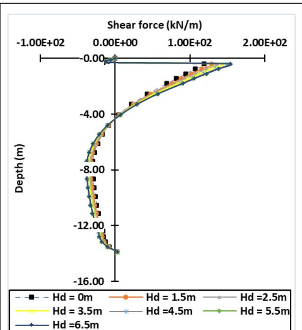
Figure 18: S.F vs Depth of barrette at ( $H_c=5m$ )
