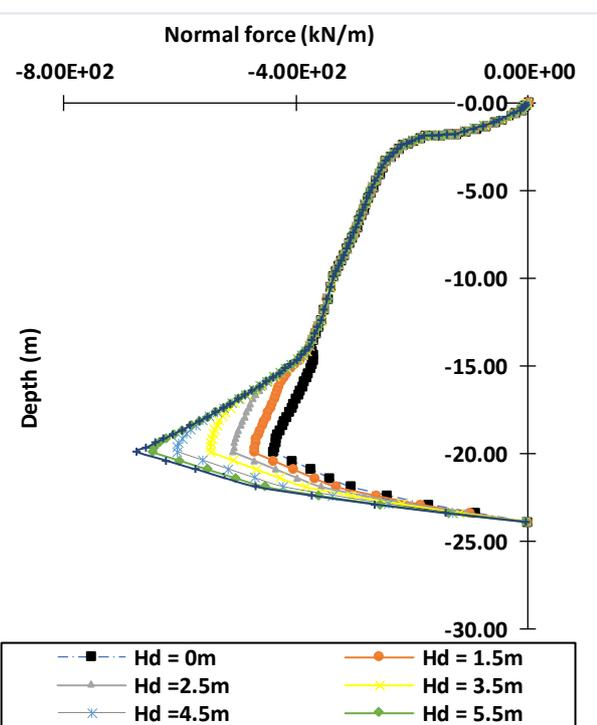
Figure 15: N.F vs Depth of DW at ( $H_e=5m$ )
