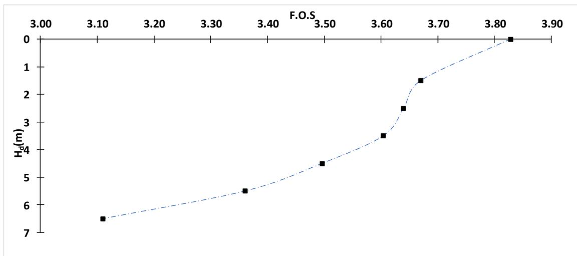
**Figure 22: F.O.S vs  $H_d$  at ( $H_e=5$ m)**
