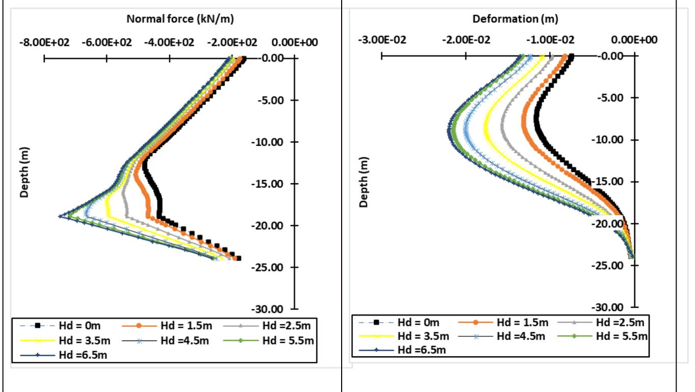
Figure 25: N.F vs Depth of DW at ( $H_e=5m$ )
