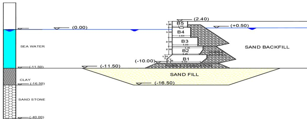
**Figure 5: Existing quay wall cross section**
