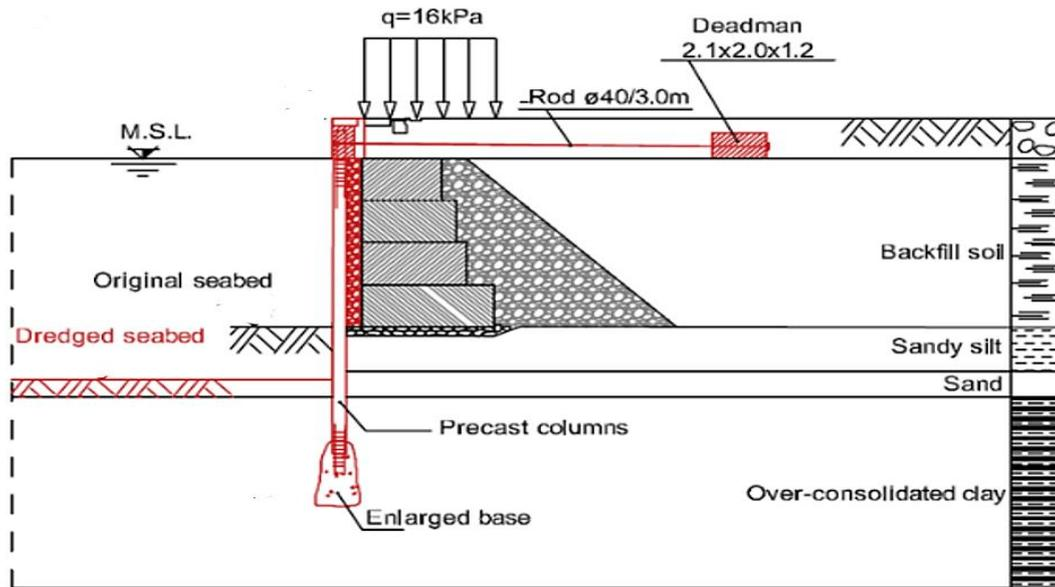
**Figure 7 : Application for first deepening technique used for upgrade of gravity quay wall in Italy (modified after Ruggeri et al., 2019)**
