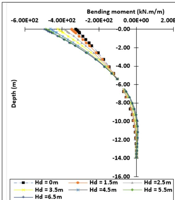
Figure27: B.M vs Depth of Barrette at ( $H_e=5m$ )
