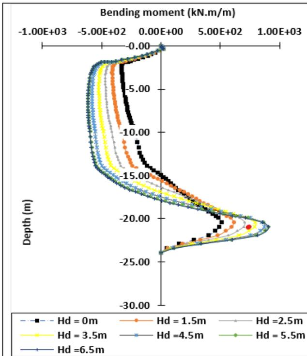
Figure 13: B.M. Vs Depth of DW at ( $H_e=5m$ )
