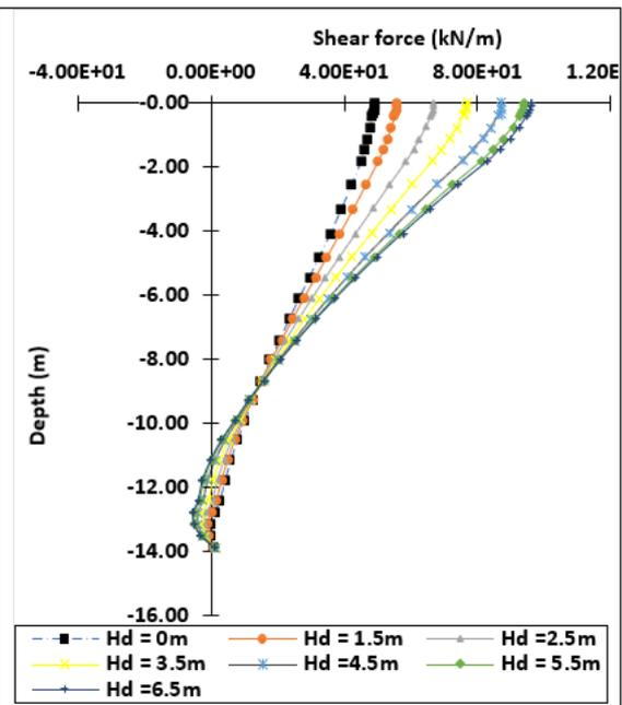
Figure28: S.F vs Depth of Barrette at ( $H_e=5m$ )
