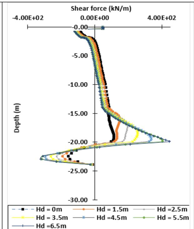
Figure 14: S.F vs Depth of DW at ( $H_e=5m$ )
