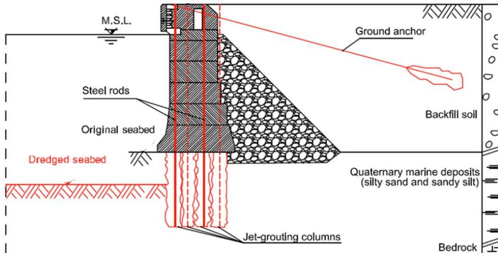
**Figure 2 San Giorgio Pier (Port of Genoa): cross-section of the quay and representation (modified after Ruggeri et al., 2019)**
