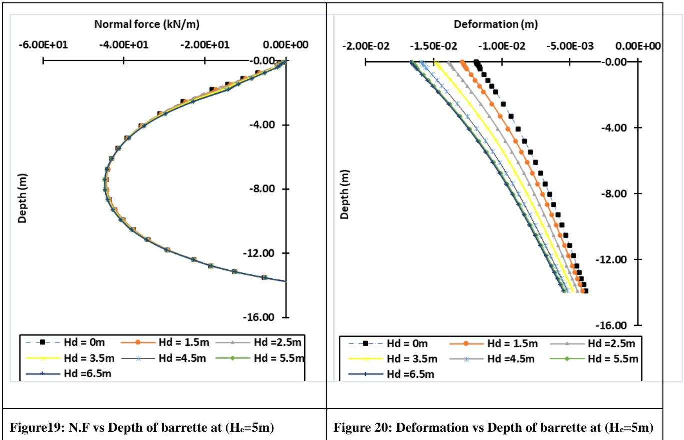
Figure19: N.F vs Depth of barrette at (H<sub>c</sub>=5m)
