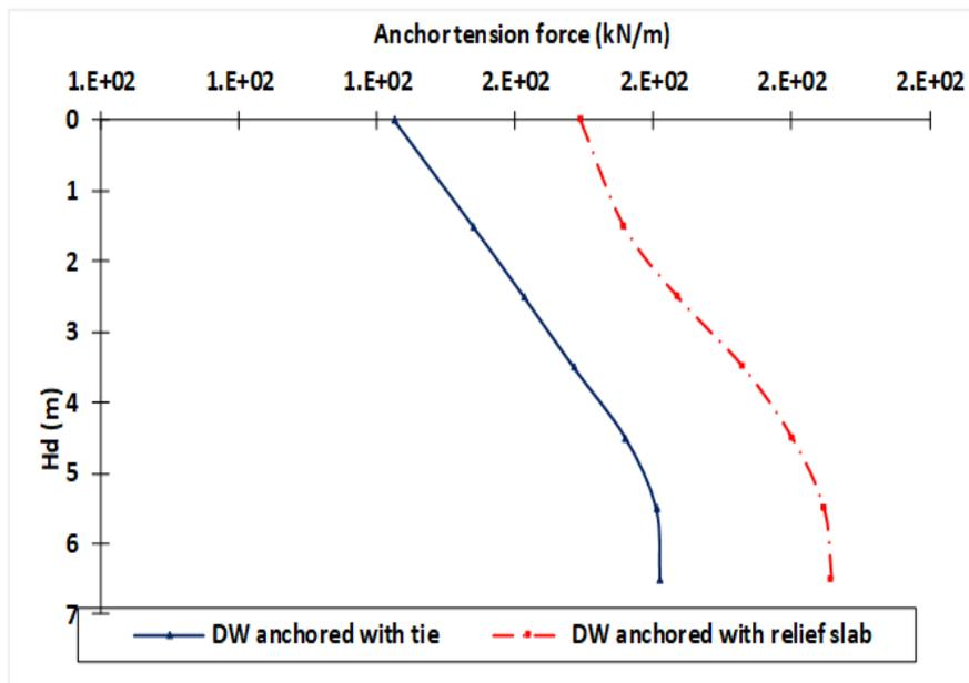
**Figure 34:  $F_a$  vs  $H_d$  at ( $H_e=5m$ )**
