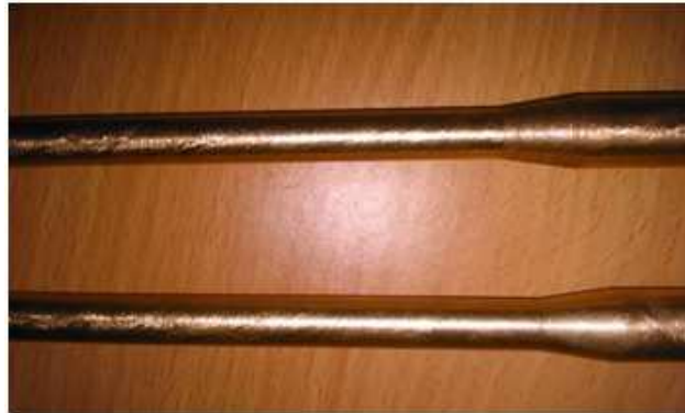
Figure 8 –Corroded fatigue test pieces of brass material
