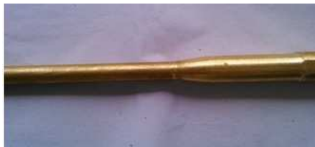
Figure 6 -Annealine fatigue test pieces of brass materials
