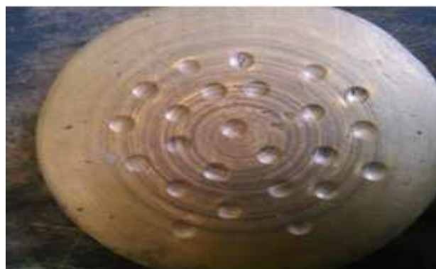
Figure 4 –Brass specimen indentation after Brinell hardness test.
