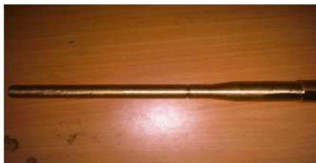
Figure 7 –Groove (1mm) fatigue test pieces of brass materials
