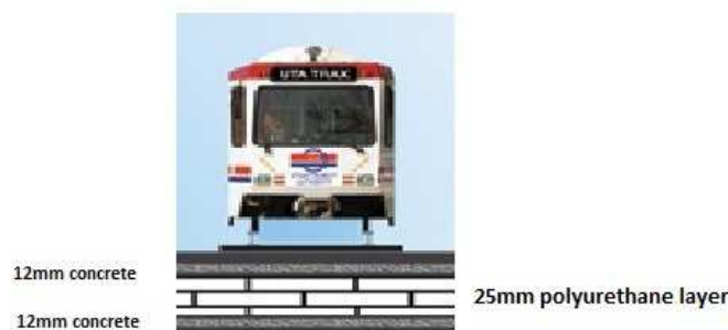
Fig 2. Polyurethane layer thickness in other areas
