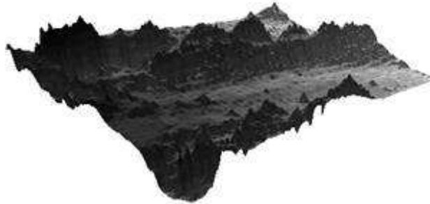
Figure 5: 3D view of the Digital Elevation Model Created using the IDW interpolation method.
