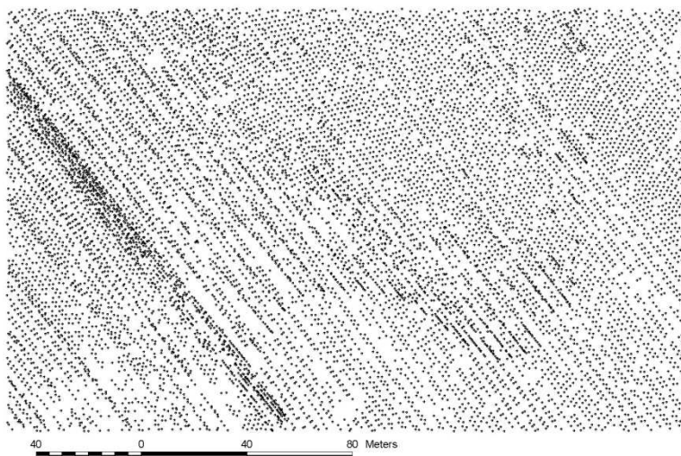
Figure 2: Row LiDAR measurements at bare lands for Gilmer county, USA in March and April 2004
