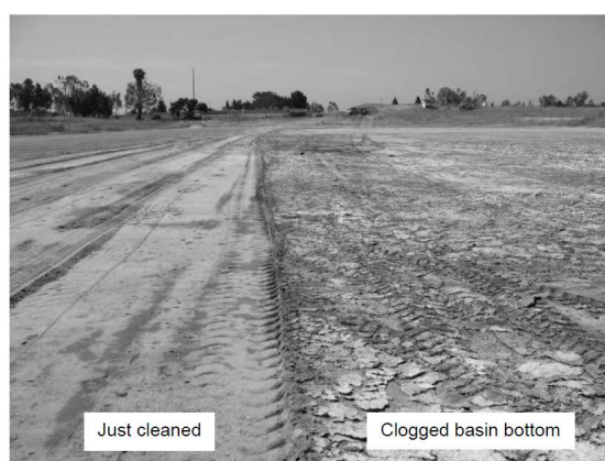
Figure 4. Clogging and cleaning layer in recharge basin operated in Orange County, California, (Bouwer, et al. 2008).
