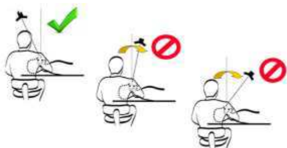
Figure 6. Optimal work light placement
